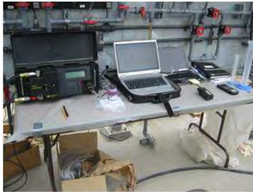
Figure 1: Fluorometer and Data Collection Setup
