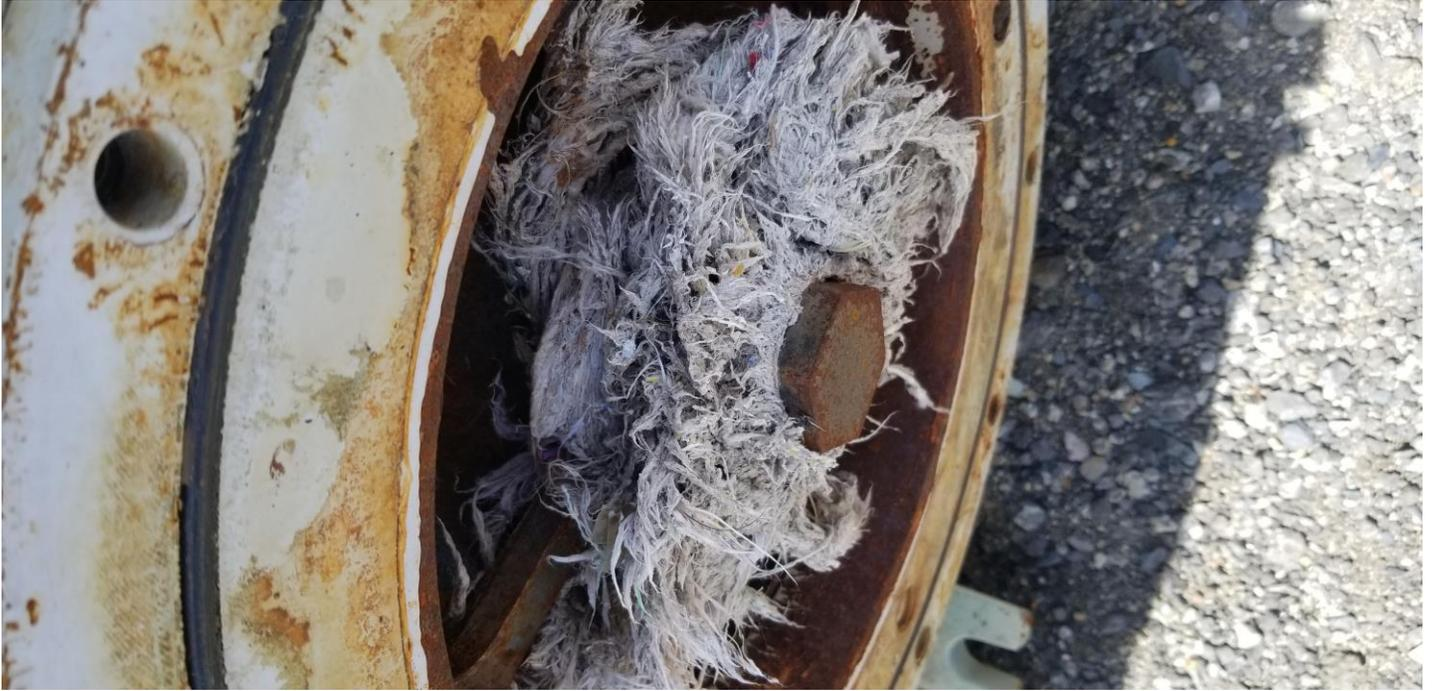
*This picture is displaying an impeller from chopper pump responsible for mixing the digester tank at the wastewater treatment plant. This impeller was no longer able to mix the digester tank efficiently due to the numerous wipes wrapped around it. This is common on District equipment.*
