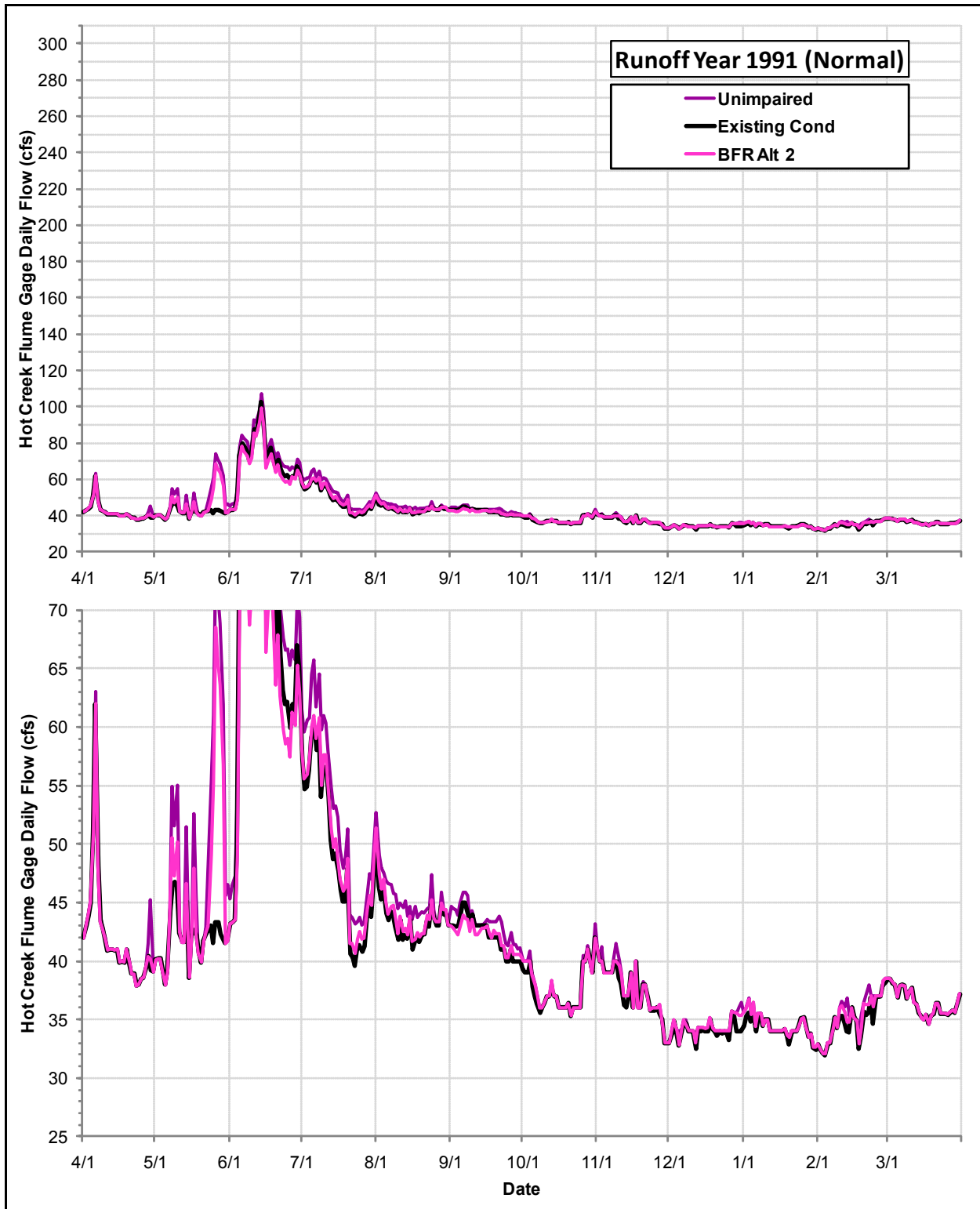
Daily Flows (cfs) at the USGS Hot Creek Flume Gage under the Bypass Flow Requirements Alternative No. 2, the Existing Condition and the Index of Unimpaired Conditions during Runoff Year 1991
